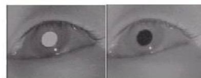
Bright (left) and dark (right) pupil images resulting from on- and off-axis illumination. The glints, or corneal reflections, from the on- and off-axis light sources can be easily identified as the bright points in the iris.
