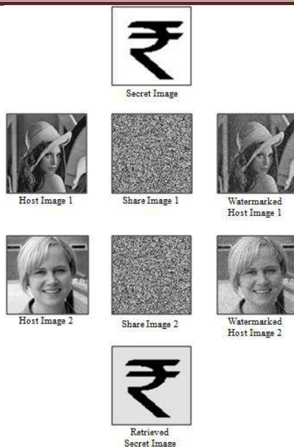
Fig. A HYBRID APPROACH- VC scheme first and digital watermarking on it.
